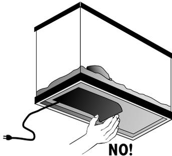
REMOVAL of the heater once attached voids all guarantees as this can easily damage the internal wire connections.
