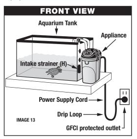
If everything is connected properly, the filter will begin to draw water up the intake tube and water will begin flowing out of the spray bar (or flow diverter). You may hear some noises upon startup that will disappear after all of the air is out of the system. It may take a few minutes for all of the air to exit the system before the filter flows at maximum capacity.
