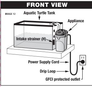
If everything is connected properly, the filter will begin to draw water up the intake tube and water will begin flowing out of the spray bar (or flow diverter). You may hear some noises upon startup that will disappear after all of the air is out of the system. It may take a few minutes for all of the air to exit the system before the filter flows at maximum capacity.
