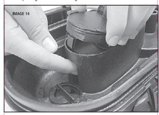
Remove the **impeller (D)** by pulling on the metal shaft.
